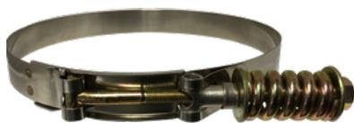
Purpose: To provide constant tension performance to compensate for the expansion and contraction when temperatures fluctuate. Provides high strength and a 360° seal. Tighten with a 7/16" wrench or hex nutdriver.
