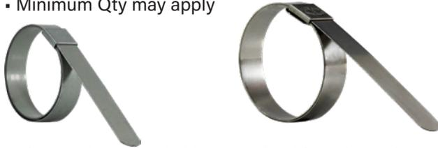
Preformed Clamps are double wrapped and formed to a given diameter. Used primarily where one end of the hose or article is free to allow the clamps to be slid over the hose end before the fitting is inserted. All clamps may be pulled down to a smaller diameter but cannot be adjusted to a larger diameter.
