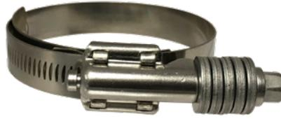
Purpose: To eliminate leaks by automatically increasing or decreasing the clamps diameter, decreasing the need for retightening. Constant torque clamps have an extended tail on the band to protect soft hose or tube from being cut.
