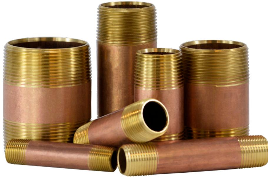
We hereby certify that to the best of our knowledge and belief the CDA 230 alloy seamless Red Brass Pipe from which our nipples are produced meet the requirements of ASTM Specifications B43 and is free of mercury contamination. The chemical analysis is 85% copper, 15% Zinc and conforms to federal Specifications WWN-351. Our brass nipples meet ANSI/ASTM B687-96 and MS51846 for standard brass nipples, and MS51872 for extra heavy brass nipples.
