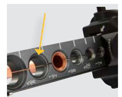
Laser etched sight gauge verifies proper flare
