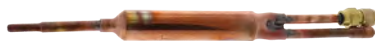
Part No. D115 Spun Copper Drier (Directional) 1/4" inlet, Cap +1/4" outlet 3/4" diameter, 3/16" process tube Recommended tonnage: (R-12)3/4 (R-22)1/2 Economy with Schrader to evacuate or charge the system, fused and scored ends
