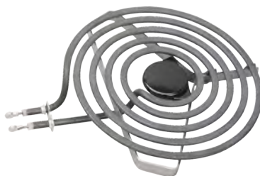
Part No. S58D21 Surface Element 8"- 5 Turn 2100W@240V
