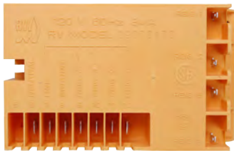
Part No. 6540S0001 Spark Module 0+4 (No manual circuits for top burner ignition, all 4 top burner circuits are individual flame sensing for automatic top burner re-ignition) Has (7) .250" & (4) .110" male terminals
