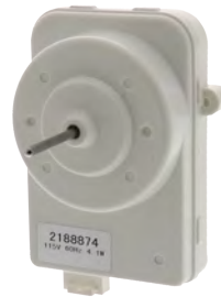
Part No. 2188874 Motor (Evaporator) 115V, 60 Hz, 4.1W, 1-1/4" shaft Replacement for Whirlpool
