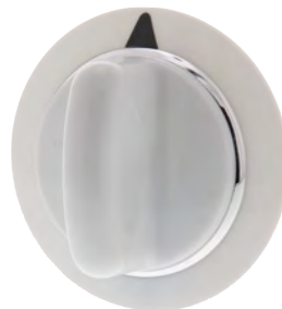
Part No. WE01X20374 Knob 2-3/4" dia., 1/8" ext. shaft, 12 o'clock flat Replacement for GE
