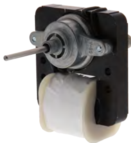
Part No. WR60X203 Motor (Evaporator) 120V, 60 Hz, .21A, 3000RPM, 1-1/2" shaft Replacement for GE
