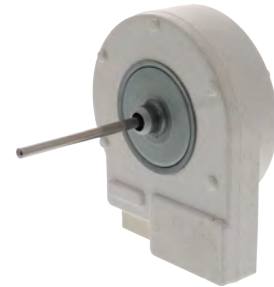
Part No. DA31-00146E Motor (Evaporator) 12VDC, 3.21W, 2520RPM, 1-1/2" shaft Replacement for Samsung
