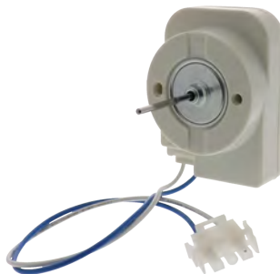
Part No. 3-60336-001 Motor (Evaporator) 115V, 60 Hz, 4.2W, 1-1/2" shaft Replacement for Whirlpool
