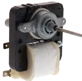
Part No. 240369701 Motor (Evaporator) 120V, 60 Hz, .135A, 3000 RPM, 1-3/4" shaft Replacement for Electrolux
