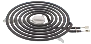
Part No. S30M2 Surface Element 8"- 6 Turn 1765W@208V 2350W@240V Replacement for GE
