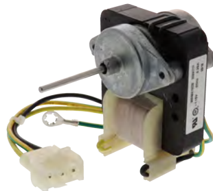
Part No. WR60X10220 Motor (Condensor) 115V, 60 Hz, .29A, 3000RPM, 1-3/8" shaft Replacement for GE
