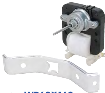
Part No. WR60X162 Motor (Evaporator) 120V, 60 Hz, .135A, 3000RPM, 1-5/8" shaft Replacement for GE
