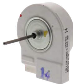
Part No. DA31-00146J Motor (Evaporator) 12VDC, 2.8W, 1920RPM, 2" shaft Replacement for Samsung
