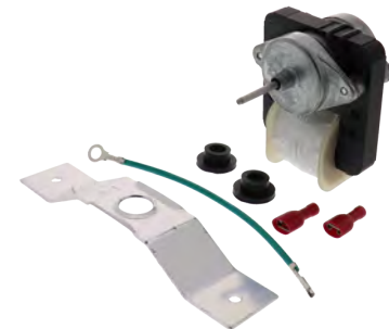
Part No. 61004888 Motor (Evaporator) 120V, 60 Hz, .21A, 3000 RPM, 1-1/8" shaft Replacement for Whirlpool
