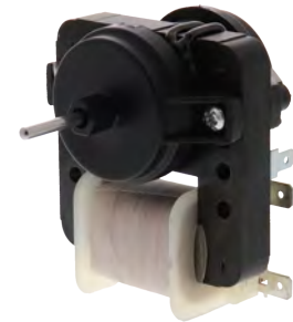
Part No. W10189703 Motor (Evaporator) 120V, 60 Hz, .135A, 3000RPM, 1" shaft Replacement for Whirlpool
