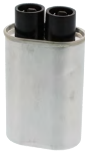
Part No. 13QBP21090 Capacitor (High Voltage) 2100V, 0.90 \mu f, 1/4" terminal size
