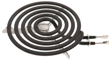
Part No. S30M1 Surface Element 6"- 5 Turn 1000W@208V 1325W@240V Replacement for GE
