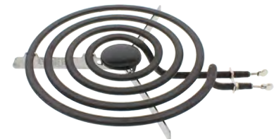
Part No. S48Y21 Surface Element 8"- 4 Turn 2100W@240V
