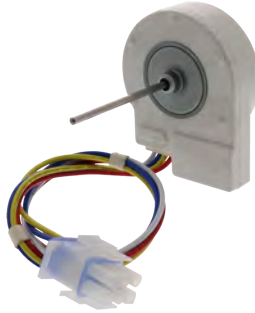
Part No. WR60X10185 Motor (Evaporator) 9.75VDC, 3.25W, 2-3/8" shaft Replacement for GE
