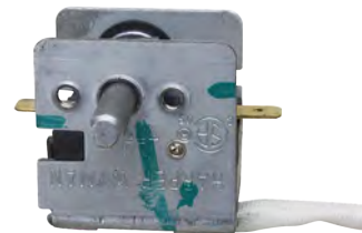
Part No. 98003984 Thermostat (Gas/Electric) 3/4" shaft, 2 terminals, single pole 120V, 5 amp, 36" capillary Replacement for Whirlpool
