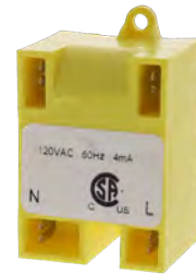
Part No. 6520S0201 Spark Module 2+0 (2 manual circuits for top burner ignition & no oven ignition circuit) Universal split terminal design suitable for: .110", .187" & .250" push on wiring
