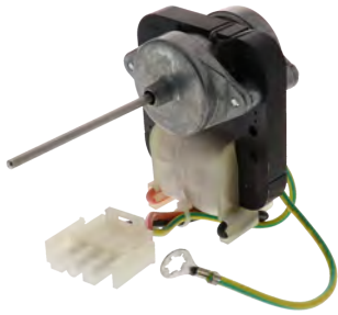
Part No. WR60X10172 Motor (Evaporator) 115V, 60 Hz, .2A, 2800RPM, 2-5/8" shaft Replacement for GE
