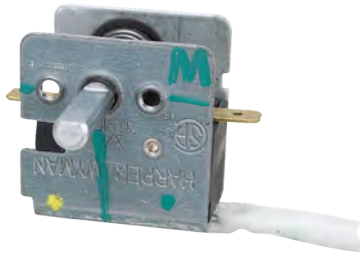
Part No. W10159016 Thermostat (Gas/Electric) 3/4" shaft, 2 terminals, single pole 120V, 5 amp, 36" capillary Replacement for Whirlpool
