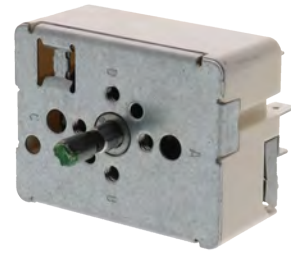
Part No. WB24T10146 Infinite Switch Current sensing type 240V, 7.2 - 9.0 amp Replacement for GE
