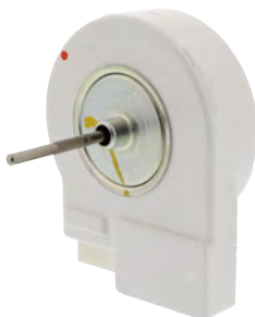
Part No. DA31-00146H Motor (Evaporator) 12VDC, 2.1W, 0.176A, 2950RPM, 1-1/2" shaft Replacement for Samsung
