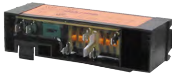
Part No. 6544S0001 Spark Module 4+0 (4 manual circuits for top burner ignition & no oven ignition circuit) Snap in mounting Has (2) .250" & (4) .187" male terminals
