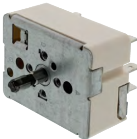
Part No. WB24T10029 Infinite Switch Current sensing type 240V, 4.4 - 7.4 amp Replacement for GE
