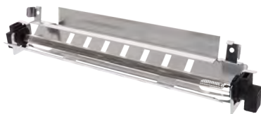
Part No. WR51X10055 Defrost Heater Quartz Tube, 725 watts @ 115V 12" tube length Replacement for GE
