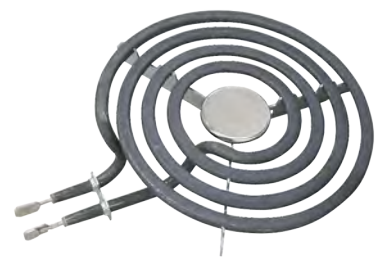
Part No. WB30T10078 Surface Element 6" - 4 Turn 1130W@208V 1500W@240V Replacement for GE
