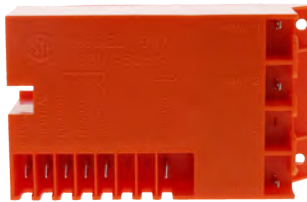
Part No. 6513S0001 Spark Module 2+1 (2 manual circuits for top burner ignition & 1 flame sensing circuit for automatic oven re-ignition) Has (6) .250" & (3) .110" male terminals
