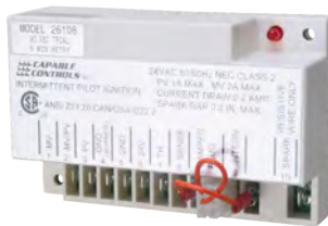
Part No. 1003 Ignition Module 24VAC, 50/60 Hz Prepurge: 1 sec. 90 sec. trial, 5 min. retry Universal Replacement
