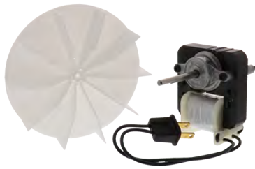
Part No. M550 Motor (Vent Hood) 0.55 amps, 3000 RPM 1-3/4" shaft, CCW Rotation
