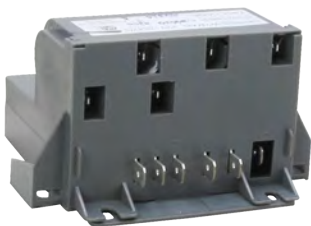
Part No. 6547S0001 Spark Module 4+1 (4 manual circuits for top burner ignition & 1 flame sensing circuit for automatic oven re-ignition) Has (6) .250" & (5) .110" male terminals
