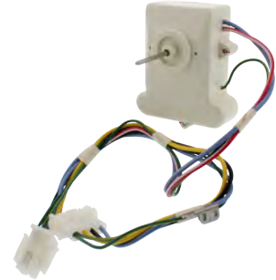
Part No. 242219204 Motor (Evaporator) 115V, 60 Hz, .33W, 2600RPM, 1-3/4" shaft Replacement for Electrolux
