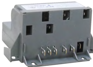
Part No. 6549S0001 Spark Module 2+1 (2 manual circuits for top burner ignition & 1 flame sensing circuit for automatic oven re-ignition) Has (6) .250" & (3) .110" male terminals
