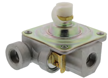
Part No. 316091706 Pressure Regulator 1/2" x 1/2" NPT 4"/10" convertible, Set at 4" natural gas Includes shut-off valve Replacement for Electrolux
