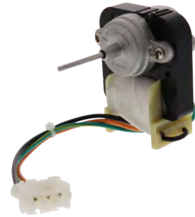
Part No. WR60X10168 Motor (Condensor) 115V, 60 Hz, 11W, .193A, 2200RPM, 1-3/4" shaft Replacement for GE
