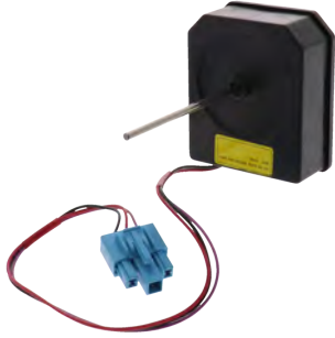
Part No. 4681JB1029B Motor (Evaporator) 13V, 150mA, CCW, 2-3/4" shaft Replacement for LG
