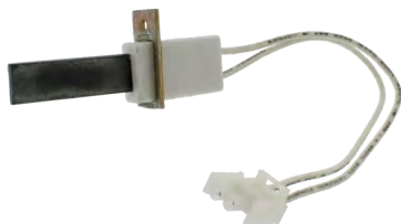
Part No. 644424 Igniter (Oven) 8-1/2" lead wires 1-1/2" ceramic block
