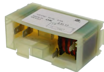
Part No. 6545S0001 Spark Module 2+0 (2 manual circuits for top burner ignition & no oven ignition circuit) Snap in mounting Has (2) .250" & (2) .187" male terminals
