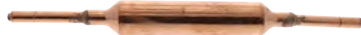
Part No. D109 Spun Copper Drier (Non-directional) 1/4" inlet, 1/4" outlet, 3/4" diameter Recommended tonnage: (R-12)3/4 (R-22)1/2 Economy with extended and fused ends
