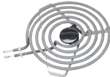
Part No. S58D26 Surface Element 8"- 5 Turn 2600W@240V
