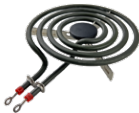
MP15YA SURFACE ELEMENT 4D6 1500W 208/240V, 1125/1500W, 6" diameter, 4 turns, 'Y' base.
