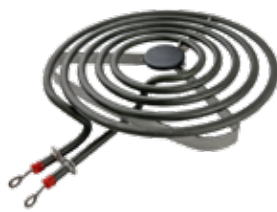
MP26MA SURFACE ELEMEN 5D8 2600W 208/240V, 1950/2600W, 8" diameter, 5 turns, 'D' base.
