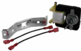
WR60X162CM EVAPORATOR FAN MOTOR 120V, .16A, 11W, 60Hz, 3000 RPM. Fits GE built refrigerators.
