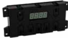
316455400CM OVEN CONTROL 7 Button Control Board. Fits Electrolux Electric ranges.
