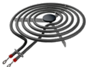
MP21YA SURFACE ELEMENT 5T8 2100W 208/240V, 1575/2100W, 8" diameter, 5 turns, 'Y' base.
