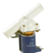
11051401CM PURGE VALVE - 240V 240V, 60Hz coil, 0.715 outlet, 0.625 inlet body. Fits Scotsman Ice Machines. Replaces Horton 560/240CDC.
