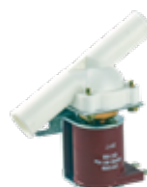
11051402CM PURGE VALVE - 120V 120V, 60Hz coil, 0.715 outlet, 0.625 inlet body. Fits Scotsman Ice Machines. Replaces Horton 560CDC.
