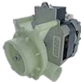
WD26X10053CM PUMP & MOTOR ASSEMBLY 115V, 60Hz, 1.5A, 3200RPM motor pump assembly. Fits newer GE dishwashers.
