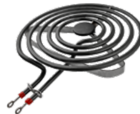
MP21MA SURFACE ELEMENT 5D8 2100W 208/240V, 1575/2100W, 8" diameter, 5 turns, 'D' base.
