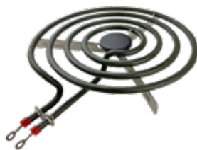
SP21YA SURFACE ELEMENT 4T8 2100W 208/240V, 1575/2100W, 8" diameter, 4 turns, 'Y' base.
