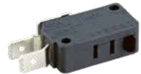
496CM MICRO SWITCH 125/250V, 15A, SPDT, 1/4" terminals. Fits many microwave models.
