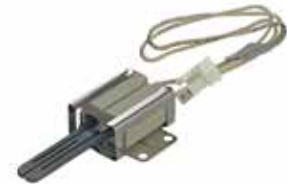
316489403CM RANGE IGNITER 3.2 - 3.6 amp, 1 1/4" block, open cage, with 16" lead. Fits Electrolux gas ranges.
